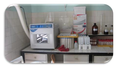
The microwave equipment for digestion soil and plant samples
