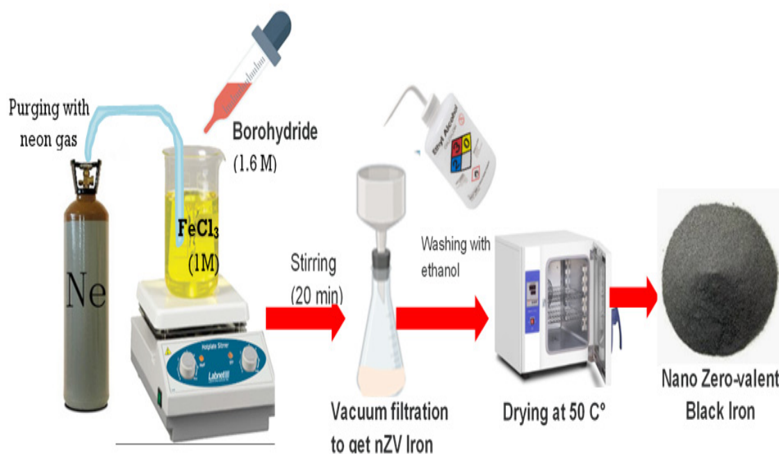
Fig. 1. Production of nano zero-valent iron (nZVI) by the reductive precipitation process using borohydride as a reducing agent, neon gas was used to keep the reductive environment. Precipitated nZVI was dried at 50 C° then kept under a thin layer of ethanol to prevent oxidation
