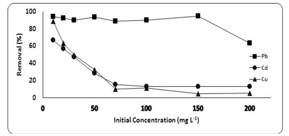
Fig. 5. Effect of solution initial metal ion concentration (mg L-1) on removal of the PTEs lead, Cadmium and Copper from their aqueous solutions using Microcrystalline cellulose MCC.
