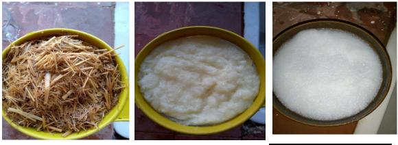
Acidified RS (1% H<sub>2</sub>SO<sub>4</sub>)/45 min
